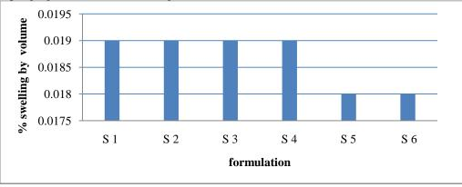
Crosslink density: Crosslink density is measure by use the florry huggins equation with the swelling data. Also in graph shows crosslink density increase with silane Si-69 uses.
